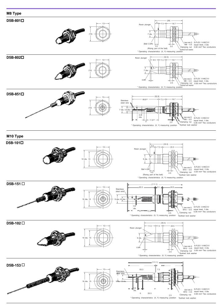
Note: 1. Unless otherwise specified, a tolerance of  $\pm 0.4$  mm applies to all dimensions. 2. The threads of the case are not standard; 0.5-mm pitch. Therefore standard tapping to the case is not possible for mounting.
